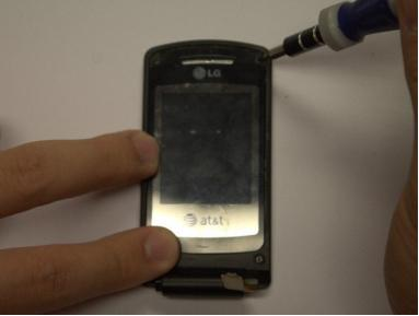
Use the small Phillips-head screwdriver to remove four 3mm screws exposed during steps 1 and 2.
