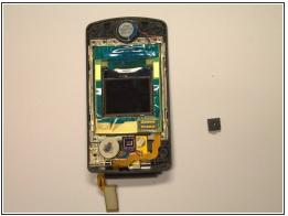
Rotate the phone 180 degrees and locate the small black square shown in the photo. Using the tweezers, pinch the raised circular lens casing and remove.
