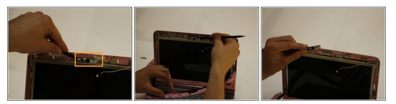
Use the spudger to pry each side of the webcam until it releases from its adhesive back.
