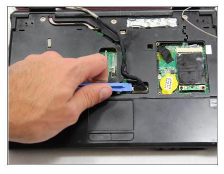
Using the plastic opening tool, pry the base of the cable connecting the screen to the motherboard upwards.
