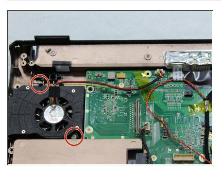
Remove the two 4.80mm Phillips #00 screws holding down the fan.
