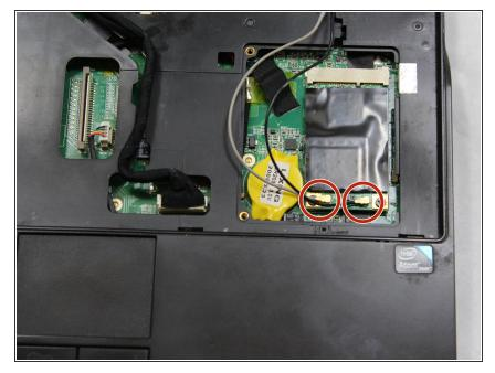
Remove the black and gray wires by gently grasping the wires where they connect to the motherboard and pulling up.
