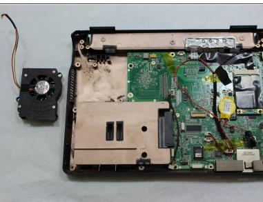
Remove the red, yellow, and black wires connecting the fan to the motherboard by placing your index finger underneath the wires where they connect to the motherboard, pinching the wires together with your thumb and index finger, and gently pulling the wires upwards.
