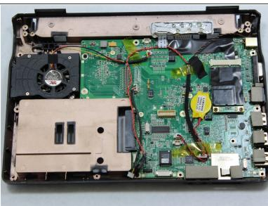
Remove the front cover plate by wedging the spudger underneath at the bottom edge of the computer and gently prying upwards while sliding the spudger around the base of the laptop.
