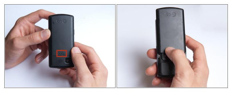
On the back of the phone, place your thumb on the three raised bumps and slide the back cover upward.
