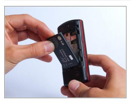
• Lift and remove the battery.
