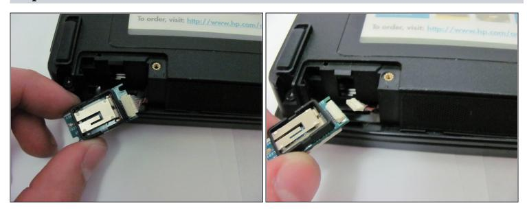
• Once the module and wire are completely outside of the casing, gently pull apart the wire from the module clip.
