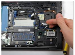
• Use a spudger or your fingernails to lift up and unclip the two gold connectors on the top of the wireless card.
