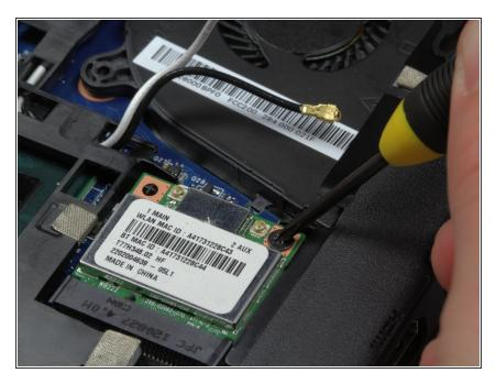
Unscrew the black #0 3mm Phillips screw at the top right of the wireless card.
