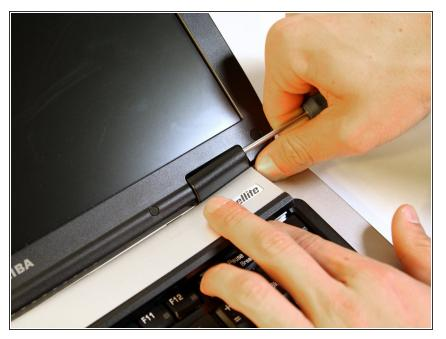
Using a screw driver for assistance, pop open the plastic cover and snap it off of the hinges. Repeat on the opposite side.
