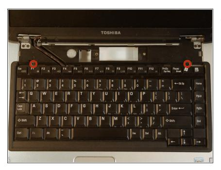
Remove the two 3mm Phillips #00 screws.
