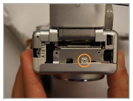
• Remove indicated screw holding front of camera in place.
