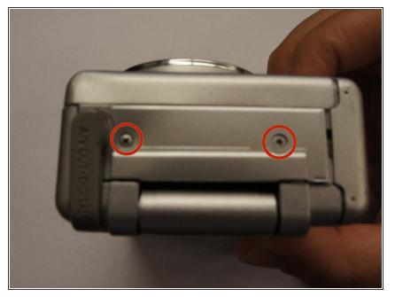
Locate and remove two screws on the same side of the camera as the marked A/V port (2x small Phillips head).
