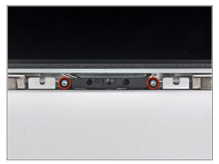
Remove the two 5.2 mm shouldered T10 Torx screws securing the camera board to the outer case.
