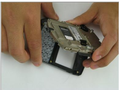
Pull the metal plate away from the front panel of the cell phone.
