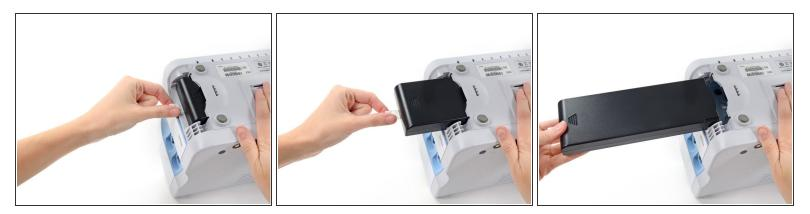
• Use the plastic label to remove the battery from its recess.
