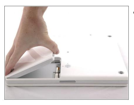
Lift the battery out of the computer.
