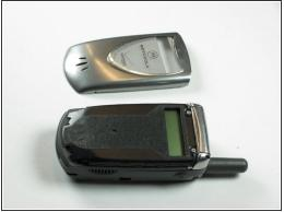
While holding the release latch, use a opening tool to help you slide off the front cover.
