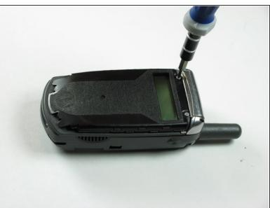
Remove the two Philips screws at top of phone with a #1 Philips screwdriver.
