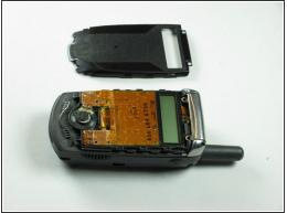
• Use a opening tool to gently pry off black cover, revealing the internal LCD display.
