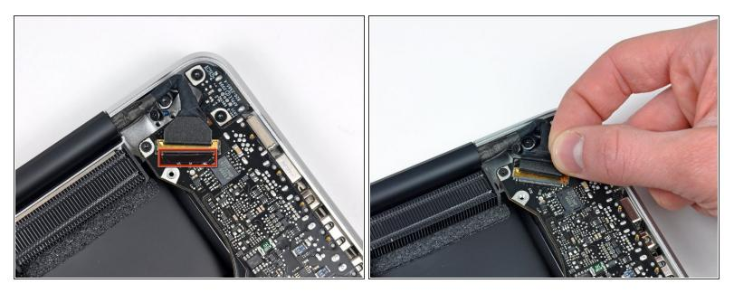
• Grab the plastic pull tab secured to the display data cable lock and rotate it toward the DC-in side of the computer.
