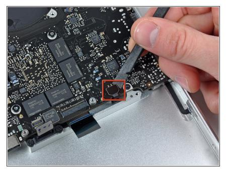
• Use a spudger to pry the battery indicator ribbon cable connector up off the logic board.
