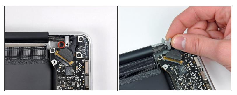
• Remove the single 7 mm Phillips screw securing the display data cable retainer to the upper case.
