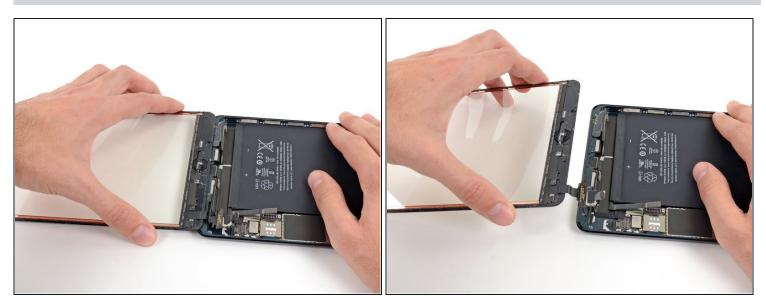
• Lift and remove the front panel from the iPad.
