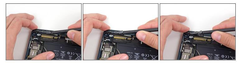
• Use the flat end of a spudger to loosen the foam adhesive holding the GPS antenna to the right speaker.
