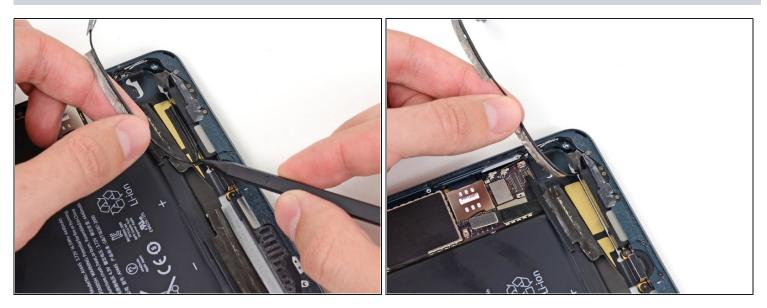
• Use the tip of the spudger to pry the antenna cable tape up from behind the right speaker as well.
