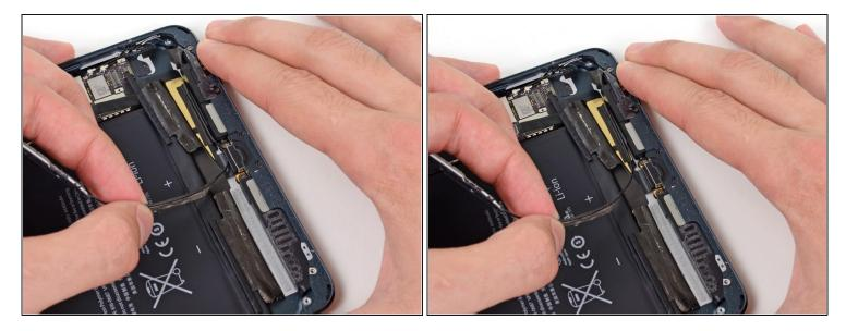
• Pull the antenna cable from the slot behind the Lightning connector.
