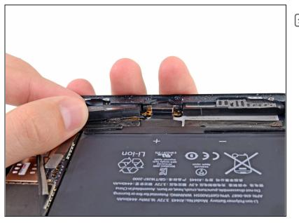
During reassembly, make sure the two speaker contacts are placed above and below the screw hole on the Lightning connector.
