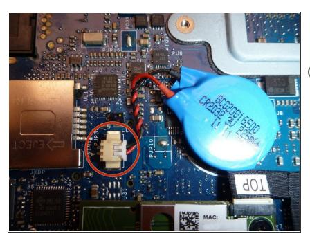
This is the BIOS battery for internal configuration and clock. If you have problems with it, remove it by disconnecting it from the motherboard.
