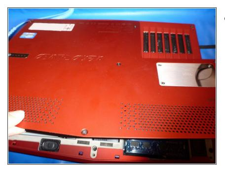
Lift the bottom cover and remove it.
