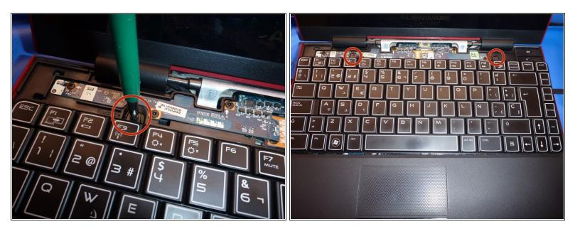
Remove the two screws to release the keyboard.
