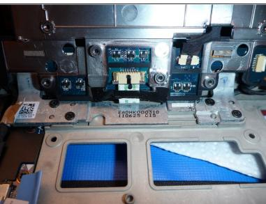
(i) Here's a top and bottom view of the board with the power on switch and LED status.
