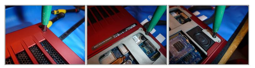
Remove the chassis screws.
