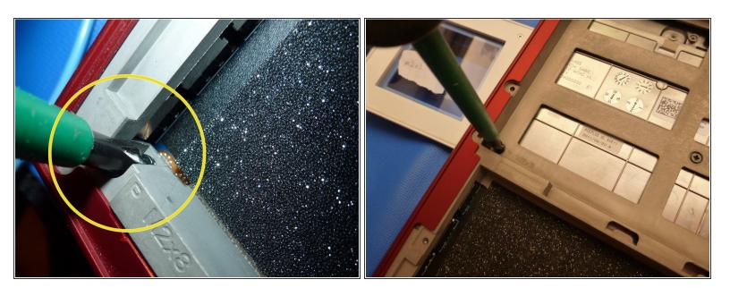
The screw marked with a yellow circle is near the hard drive bay.
