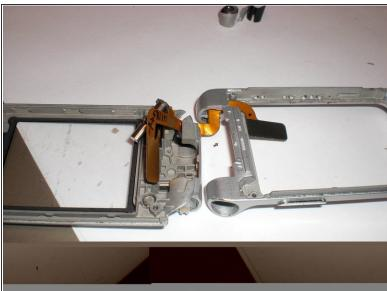
• Push in the white thing in the middle, it's spring-loaded, and pull the frame halves apart.
