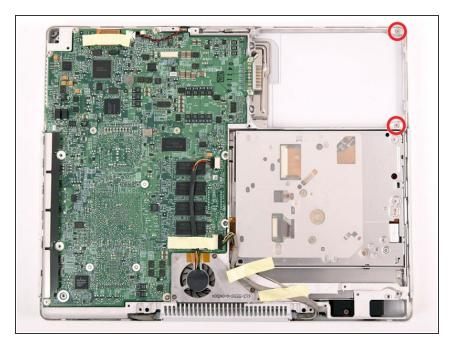
• Remove the two Phillips screws from the battery compartment.
