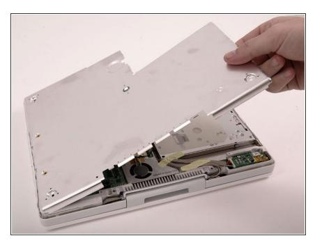
• Lift the bottom shield off.
