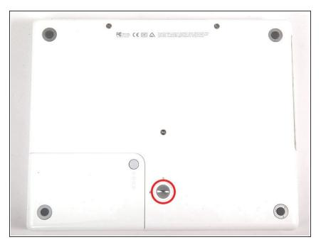
• Use a coin to rotate the battery locking screw 90 degrees clockwise.
