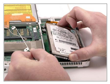
• Lift the hard drive up and remove the metal bracket, then carefully lower the hard drive back into its compartment.
