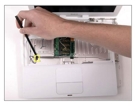
Lift the upper case off completely and disconnect the multicolored speaker cable from the logic board.
