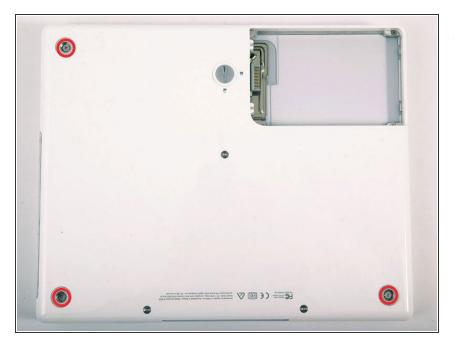
Remove the three newly-revealed Phillips screws.
