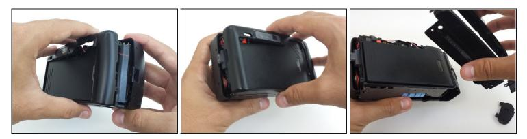
• Loosen the back cover from both the left and the right sides of the camera. Take off the back cover.
