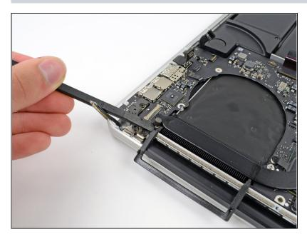
Use the flat end of a spudger to carefully pry off the rubber screw cap on the raised screw head near to the MagSafe 2 connector.
