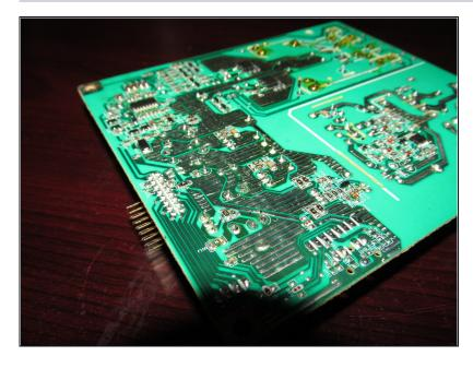
After verifying there are no cold solder joints, clean the board.
