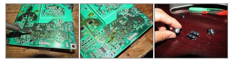
• Once the polarity is verified, solder the capacitors in. After installation, cut off any excess lead.
