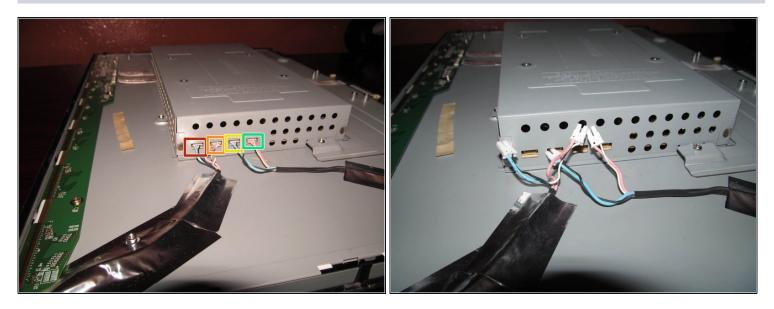
• Disconnect the CCFL cables from the power supply board.
