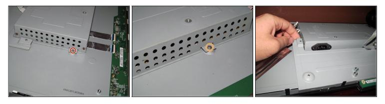
The lower shield does not have to be removed. However, it will make disassembly easier.
