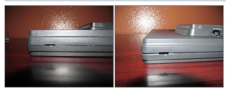
*i* If the monitor has never been serviced, a flathead screwdriver may help *at the expensive of damaging the plastic.*
