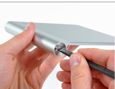
Unscrew the battery door by turning the screw counter-clockwise with a flat edge screwdriver, coin, plastic opening tool, or fingernail.
