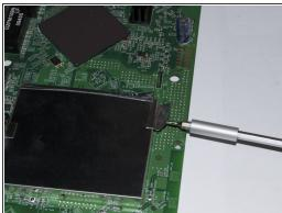
Remove the shield for microwaves circuit
