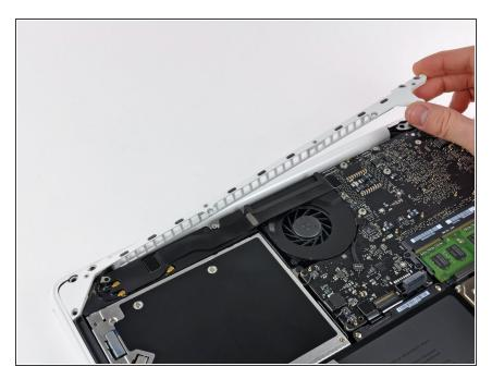
• Carefully lift the rear vent out of the upper case.
