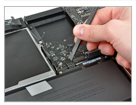
Use the flat end of a spudger to pry the trackpad ribbon cable connector up off the logic board.
