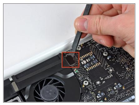
Use the flat end of a spudger to pry the AirPort/Bluetooth ribbon cable up off the logic board.
