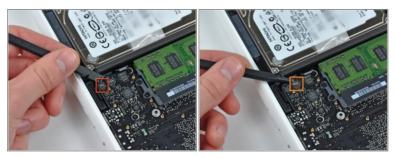
• Use a spudger to pry the left speaker connector and microphone connector up off the logic board.
