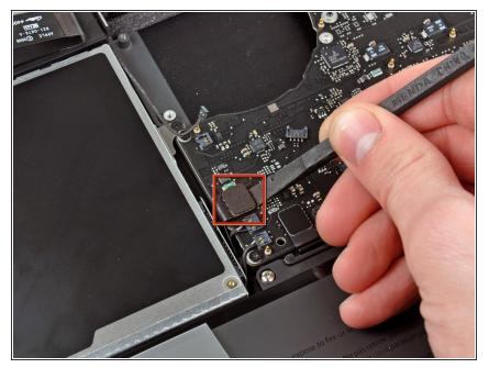
• Use the flat end of a spudger to pry the optical drive connector up off the logic board.
