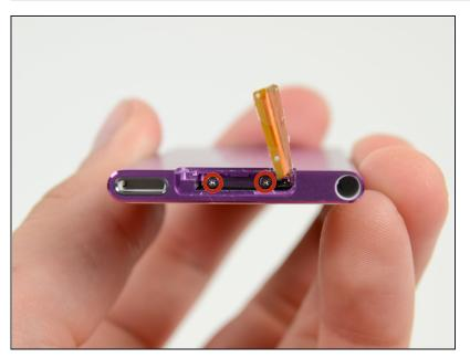
Remove the two 2 mm Phillips #000 screws from the bottom of the case.
