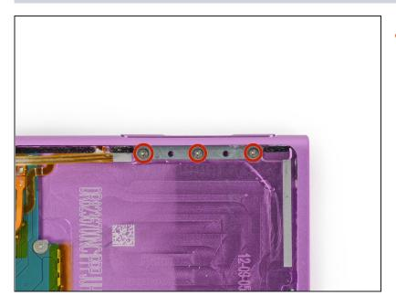
Remove the three 1.4 mm Phillips #000 screws securing the volume control button assembly to the rear case.
