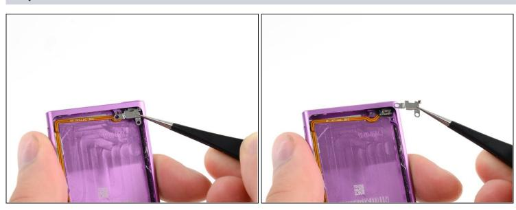
• Remove the sleep/power button bracket from the rear case.
