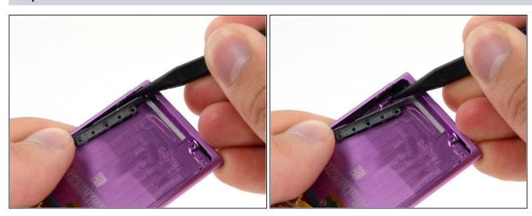
Use the pointed end of a spudger to pry the volume control button assembly away from the edge of the case.
