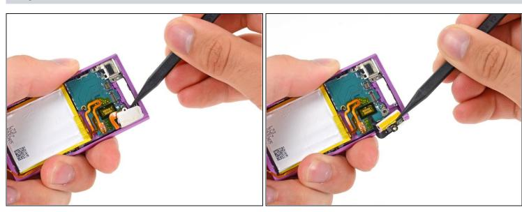
• Use a spudger to pry the headphone jack off of the adhesive holding it to the rear case.
