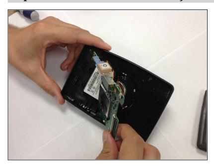
Remove and disconnect the motherboard and battery from the back panel.
