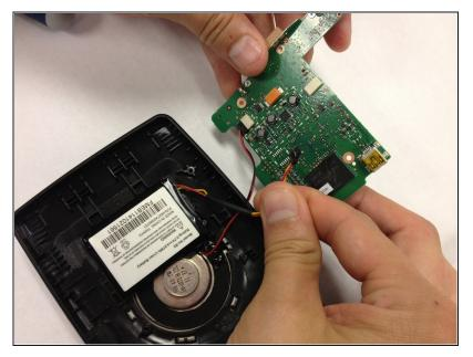
Attach the motherboard and battery to the new back panel.
