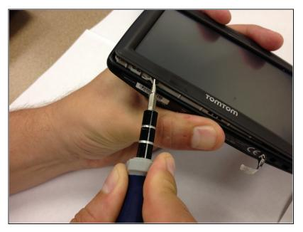
• Use a flat edge screwdriver to pry open the faceplate.
