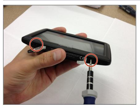
Unscrew the two T5 screws using the T5 Torx Screwdriver.
