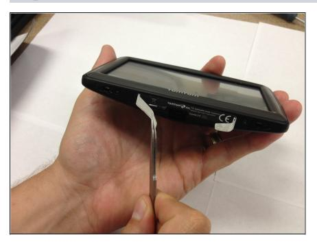
Re-apply the label edges back down to cover the screws.
