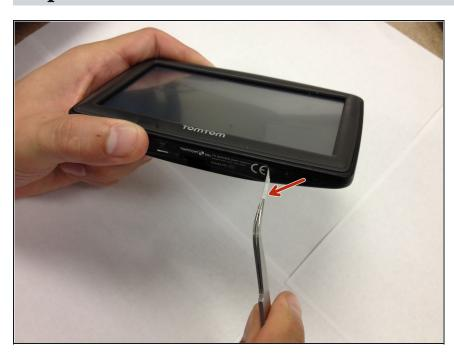
Peel back the sticker, using the tweezers on the bottom of the device to reveal the two screws.
