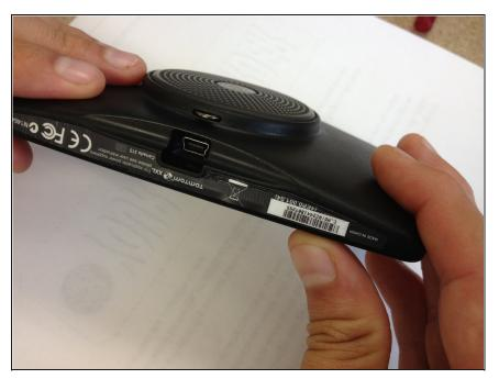
Using two hands, hold both ends of the device and snap the two plates together.
