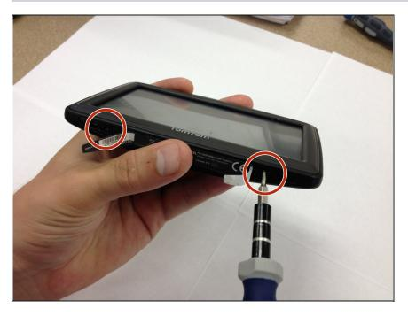
Re-insert the two T5 screws and tighten.
