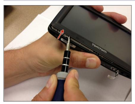
Insert the flat head screwdriver into the edge of the device. Using it as a lever, carefully pry the face-plate up.
