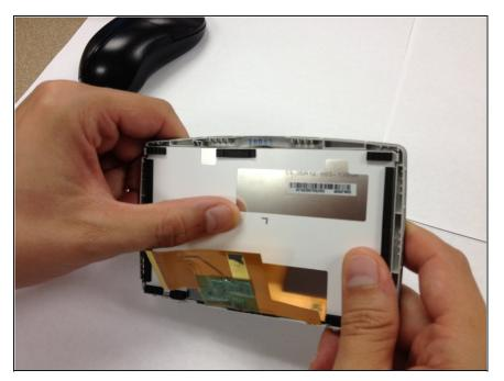
Insert the new screen into the face-plate.
