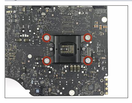
Remove the four 12 mm T10 shoulder screws from the spring plate behind the CPU.
