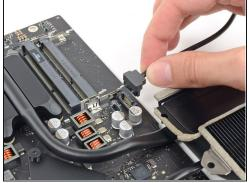
• Disconnect and remove the SATA data and power cables from the logic board.
