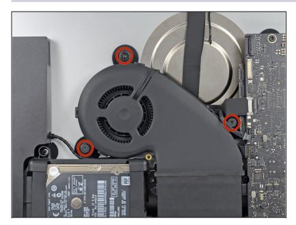
• Remove the three 12.3 mm T10 shoulder screws securing the fan to the rear enclosure.
