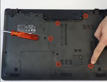
Using a Philips #1 screwdriver, unscrew the 5 screws securing the cover.
