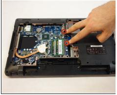
• Using a Phillips #1 screwdriver, remove all 16 screws that secure the entire cover.
