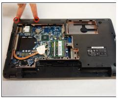
• Using the Phillips # 1 screwdriver, remove the 16 screws that secure the cover.
