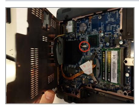
Since the ventillator is mounted under the cover, its power supply cable must first be disconnected so that the cover can then be completely removed.
