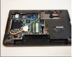
Using a Phillips #1 screwdriver, remove all 16 screws that secure the entire cover.
