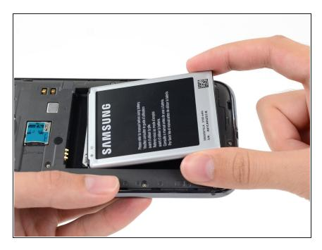
• Remove the battery from the midframe.
