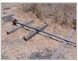
Carefully lower the riser main, horizontally, and place it in a sanitary place, preferably resting above the ground, to prevent contamination.
