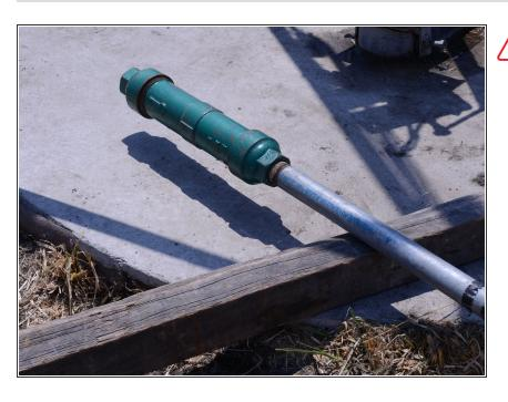
Make sure to keep the cylinder off the ground to prevent contamination.
