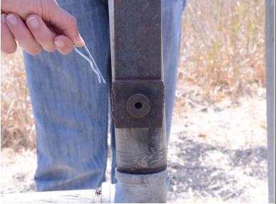
Remove the two pins connecting the handle to the slider.
