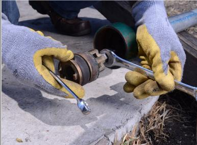
Unscrew the valve from the pump rod.
