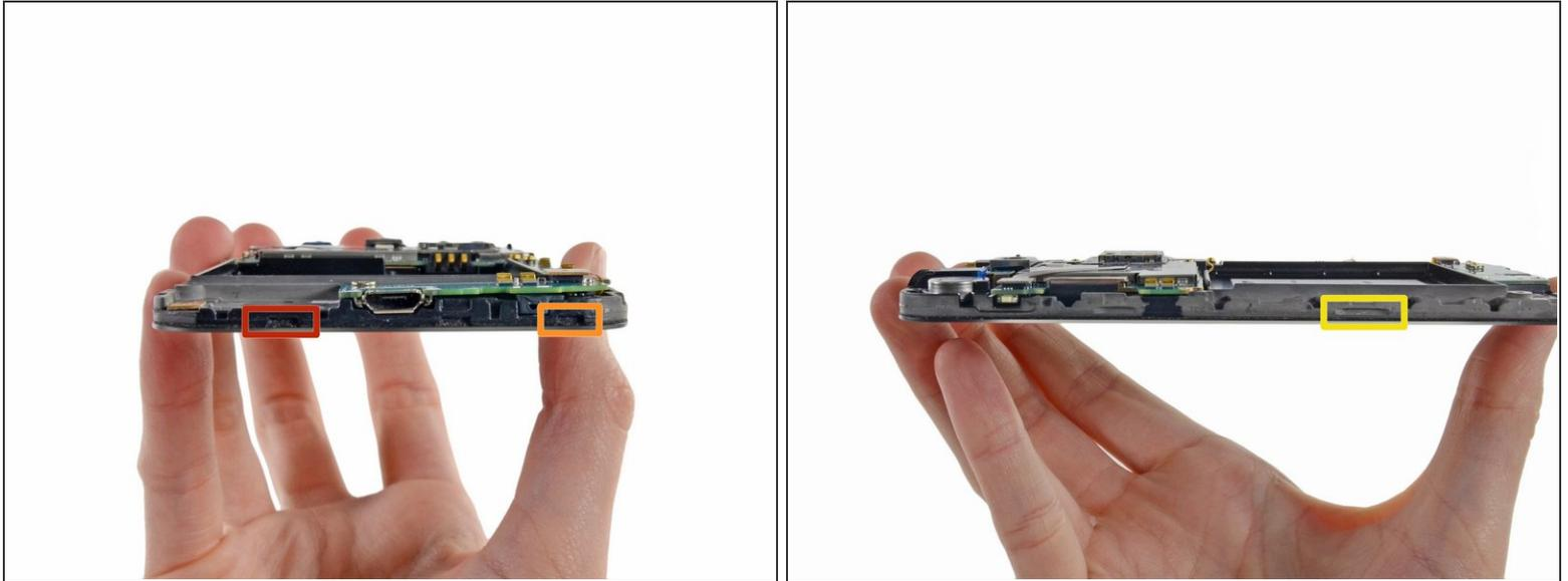
**i** Unless you pry at the right insertion points, you might have a difficult time removing the midframe. This shot of the display assembly, with display glass facing down, is meant to help you locate them.
