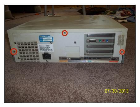
Using a Phillips screwdriver, remove the three Phillips head screws (circled in red) from the back of the computer.
