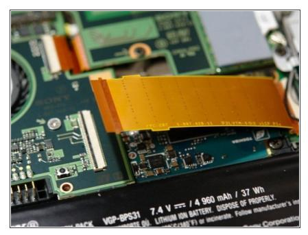
• Detach flat cable. To do so, you have to lift the black plastic bar, then release the orange ribbon.
