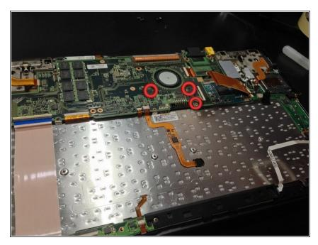
• Remove these screws to make it easier to remove the SSD.
