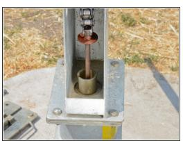
Place the spacer collar around the pump rod below the raised chain, with the beveled side down, and the flat side facing up.
