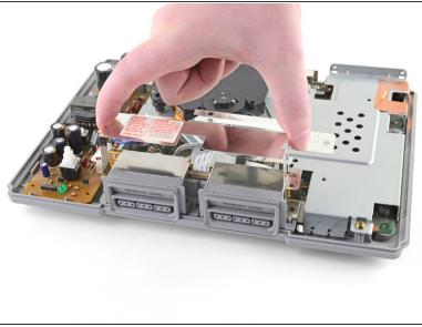
• Lift the metal shield straight up to remove it.
