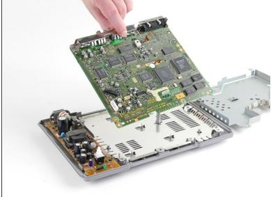
Lift the motherboard out of the bottom case.
