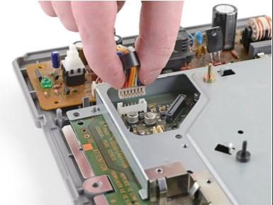
• Pull the power supply cable straight up and out of its socket on the motherboard to disconnect it.
