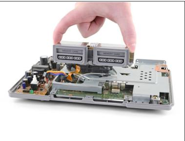
• Lift the controller ports straight up and out of the bottom case.
