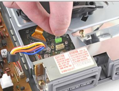
Pull the optical drive power cable straight up and out of its socket on the motherboard to disconnect it.
