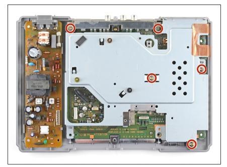
Remove the five 14 mm-long Phillips #1 screws from the motherboard's metal shield.
