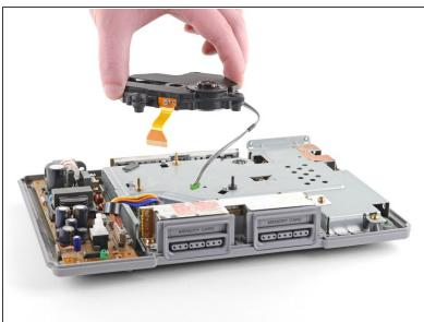
Lift the optical drive straight up to remove it.
