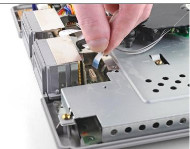
Pull the controller port's ribbon cable straight up and out of its socket on the motherboard to disconnect it.
