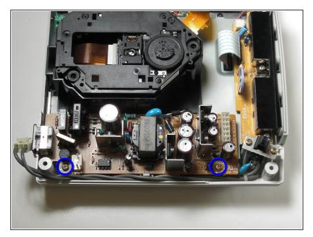
Remove the two 10mm Philips #02 screws that are fastened to the power block.
