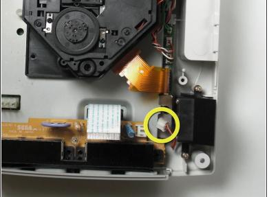
Disconnect the white fan header from the controller port.
