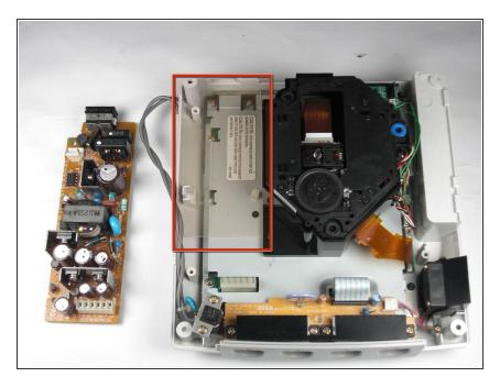
Remove the clear plastic film that is tucked between the power supply and the chassis.
