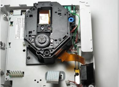
Detach the orange cable by giving it a gentle pull while wiggling the cable back and forth until it loosens from the logic board.
