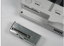
Remove the expansion bay by applying pressure to the small clip on the expansion bay while prying it away from the console.
