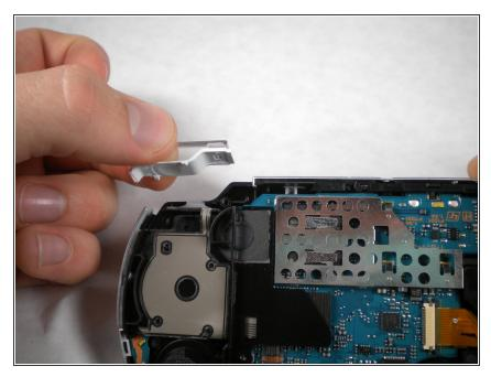
• Remove the 'L' trigger from the PSP.
