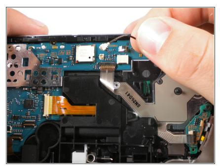
Remove the cable carefully by lifting upwards from port attached to the motherboard.
