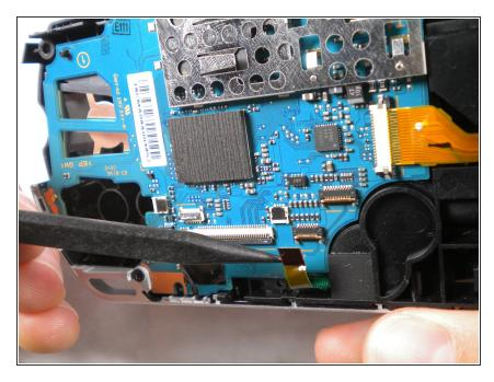
Flip up the lock and remove the ribbon cable located at the bottom edge of the PSP.
