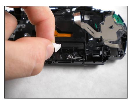
On the bottom of the back of the PSP, pull the white plastic piece out.
