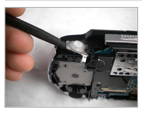
Being careful not to break the ribbon cable, use the spudger to peel the adhesive button of the the 'L' trigger off the PSP.
