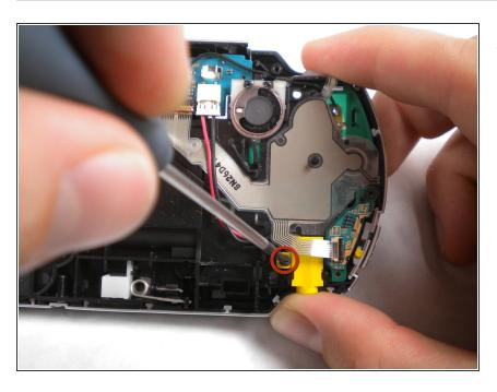
Remove the screw from the power jack.
