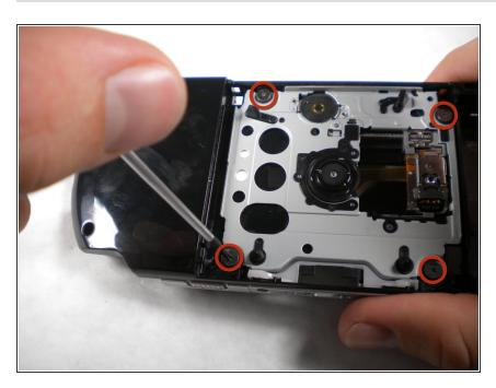
Remove the four screw from the UMD drive.
