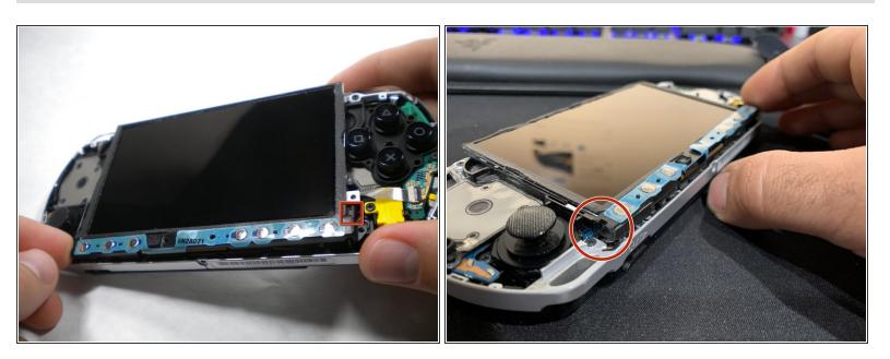
Push the homebar to the right to release the tab located on the right side of the LCD screen.
