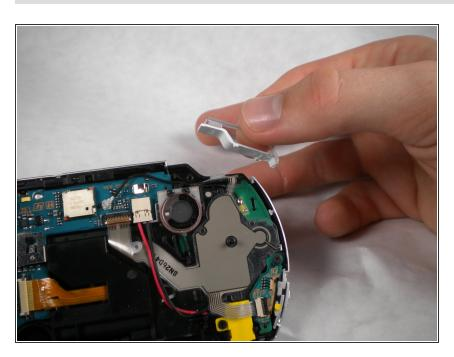
Remove the 'R' trigger from the PSP.
