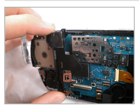
Remove the cable from the connector and remove the entire black piece from the PSP.
