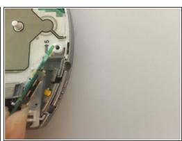
Remove the screw located at the top of the power switch panel.
