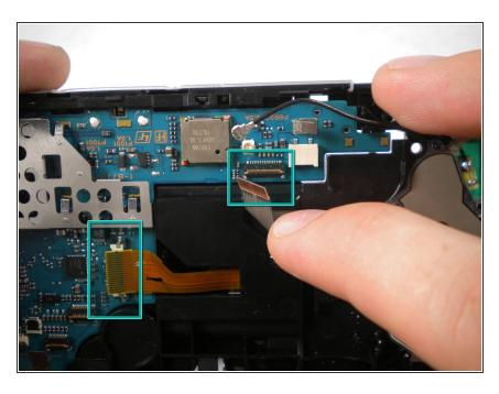
Flip up both of the locks and remove both cables as shown
