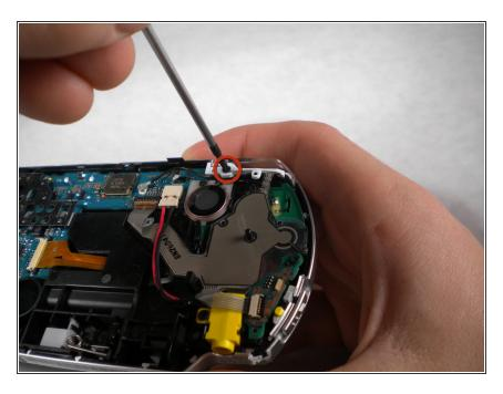
Remove the screw securing the 'R' trigger.
