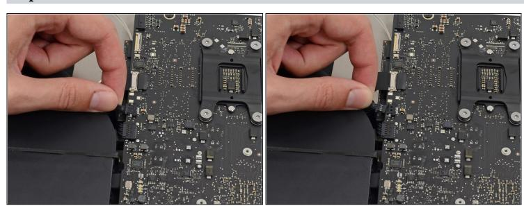
• Disconnect the fan cable connector from its socket on the logic board.
