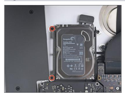
Use a T8 driver to remove the two 7.3 mm screws securing the left hard drive bracket to the rear case.
