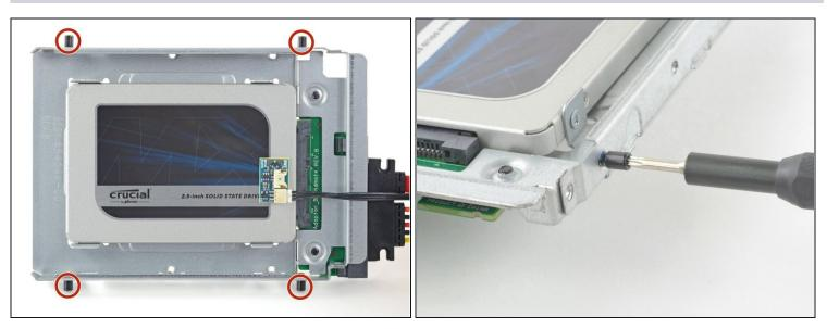
• Use a T8 driver to install the mounting pins from the old hard drive onto the sides of the enclosure.
