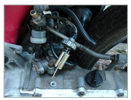
Here is the assembled throttle cable.
