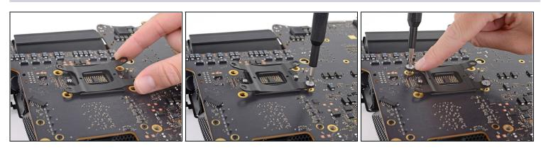
• Place the spring plate on the backing plate.
