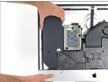
• Lift the left speaker straight up, until the power button cable is exposed (about 0.5 inches).
