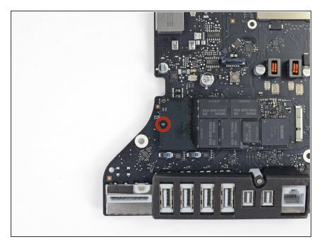
Remove the single 5.3 mm T8 screw securing the SSD to the logic board.
