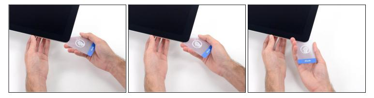
• Insert a second card into the gap between the display and frame in the top left corner.
