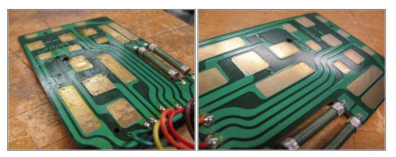
• If someone spilled soda or apple juice over the controller it may be helpful to clean the board using contact cleaner.
