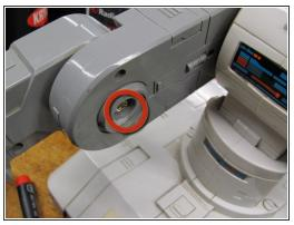
Use the knife to peel off stickers that conceal the screw holes.
