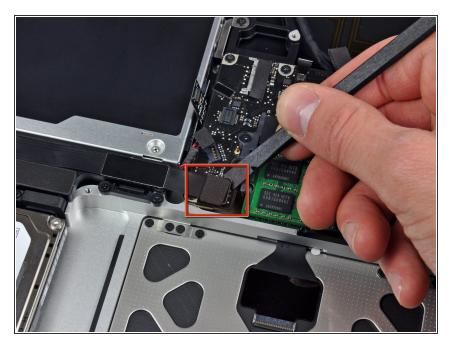
Use the flat end of a spudger to pry the hard drive/IR sensor cable connector up off the logic board.
