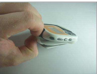
Remove the belt clip by pulling the clip casing up and away from the device starting at the top over the slightly protruding headphones jack.
