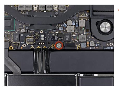
Remove the wide head 6.4 mm T6 Torx screw securing the battery connector to the logic board assembly.
