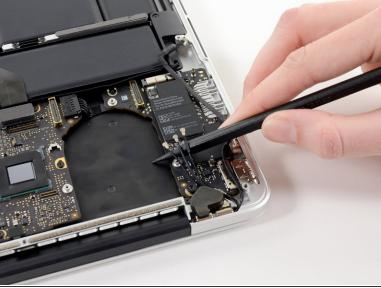
Move the antenna cables aside, clear of the AirPort board.
