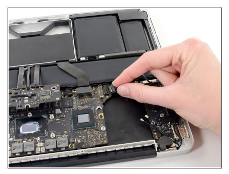
Pull the I/O board connector straight out of its socket on the logic board.
