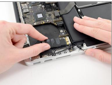
Pull the AirPort board straight out of its socket on the I/O board.
