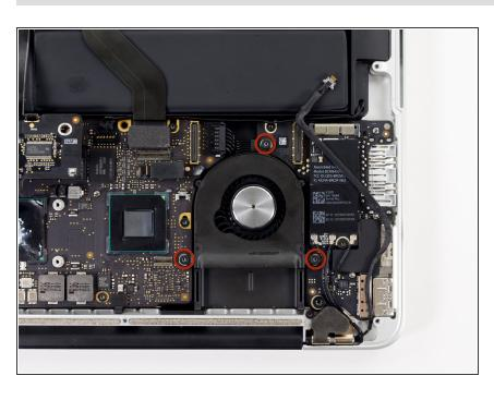
Remove the three 3.1 mm T5 Torx screws securing the right fan to the logic board assembly.
