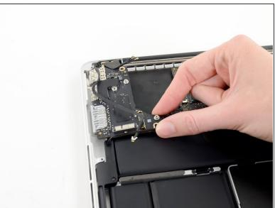
Carefully pull and remove the I/O board away from its recess in the upper case.
