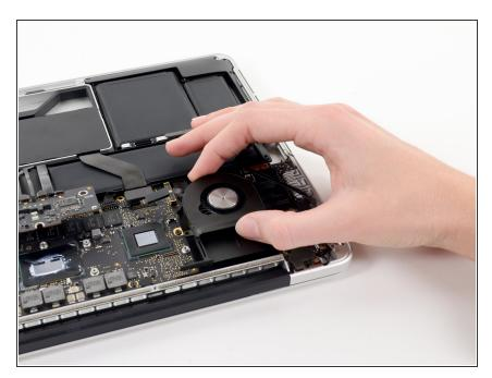
Lift and remove the right fan out of the upper case.
