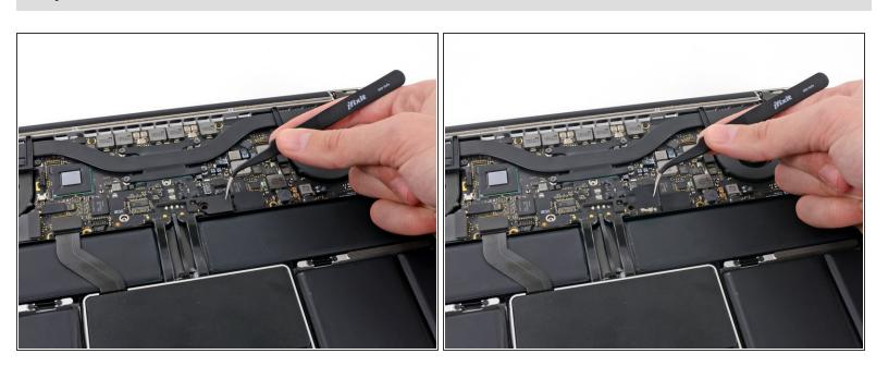
Use tweezers to remove the small plastic cover located near the bottom right of the battery connector board.
